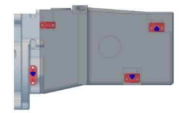
**FS.10 Transponder:** An AMB transponder must be fitted in the provided location on the rear wing upright.
