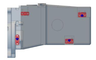
FS.10 Transponder: An AMB transponder must be fitted in the provided location on the rear wing upright.
